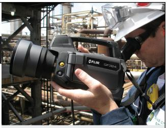
Check for hydrogen leaks from many components in a power generation facility with the GF343 while using  $CO_2$  as a tracer gas.
