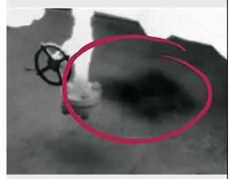
Image of gas leaking from a valve. Optical gas imaging cameras like the GF343 can be used to inspect for similar leaks in the power utility industry.
