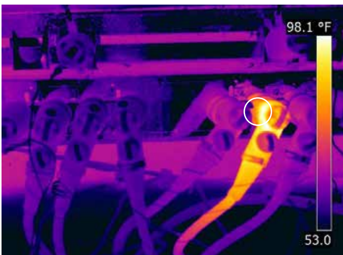
Load Break Elbow with Auto (top) and 1-Touch Level/Span (bottom)
