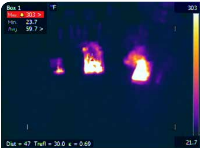
During a controlled demonstration of the Fire Rover's firefighting capabilities, the Watchdog Security team set fire to jet fuel in open metal bins. The FLIR A310f thermal camera instantly detected each fire, triggering a visual alarm (marked in red above). An operator using a laptop then aimed and released the Fire Rover's fire-fighting foam, extinguishing the fires in seconds.
